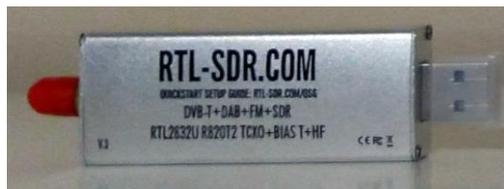
*Figure 1: Software Defined Radio - USB “Dongle” form factor*
